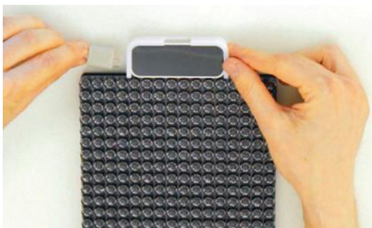
2. Ultrahaptics initial array utilizes standard automotive ultrasonic speakers. The array is driven by an FPGA. A Leap Motion 3D sensor is used to determine the range to target.
