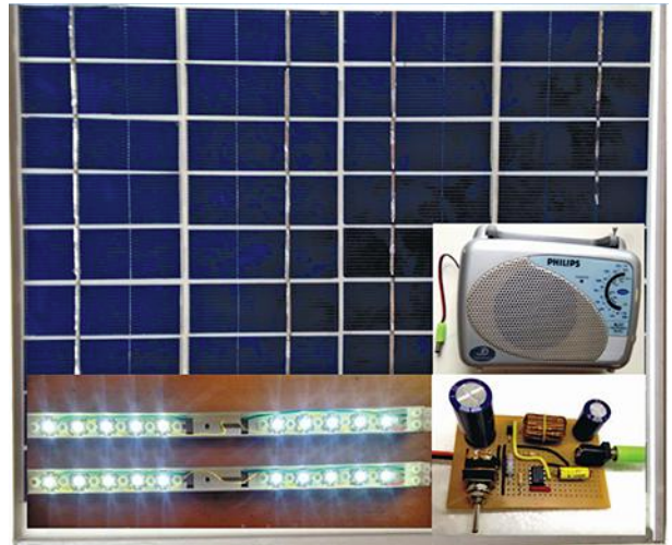
5. The day lamp can also use two PV panels, but the topology must be adjusted to avoid excessive voltage on the regulator.
