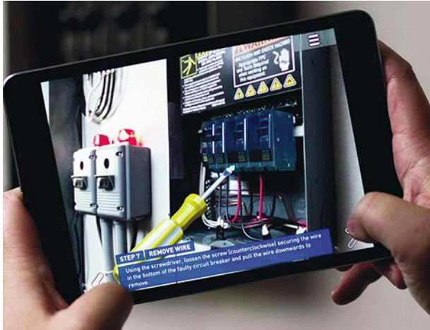
5. Scope AR's augmented-reality software can utilize devices like tablets and smartphones to add information to a scene captured by the device's camera.
