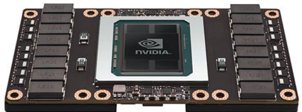
4. Nvidia's Tesla P100 GPGPU is built using chip-on wafer-on substrate technology to deliver 21 TFLOPS of 16-bit floating-point computing ideal for DNN applications.
