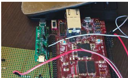
4. The Xilinx Zynq's Bank 34 T10/T11 differential pair is used to demonstrate BMC signal decoding, based on a circuit in the MicroZed Breakout Carrier Card Hardware User Guide. The photo below shows the actual setup using MicroZed (also see Ref. 4).
