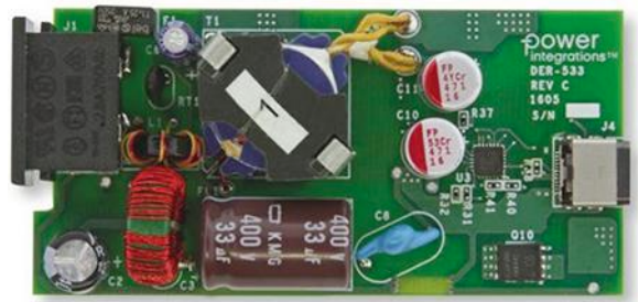
The DER-533 reference design is capable of 5-V/3-A and 9-V/2.2-A power delivery over a standard 3-A USB Type-C cable. (Courtesy of Power Integrations)
