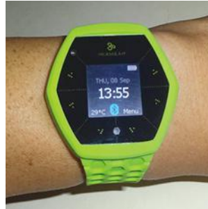
6. Hexiwear is a module that can fit into a wristband so that a user can take advantage of its portability and a heart rate monitor.
